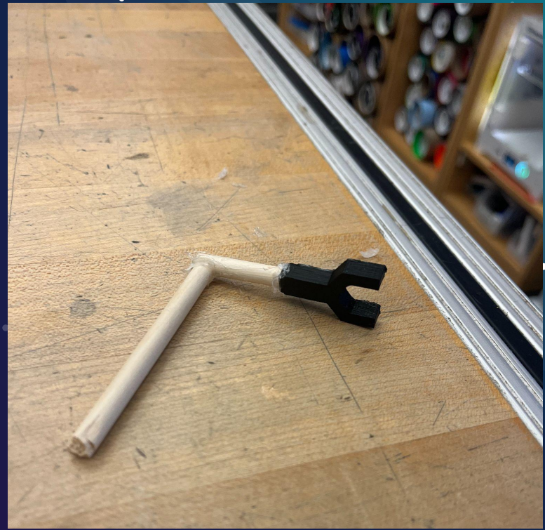
Space Wrench Rapid Prototype with printed wrench and wooden dowels glued together with hot glue
