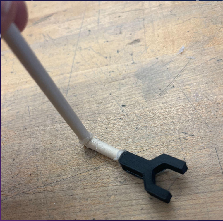
Space Wrench Rapid Prototype with printed wrench and wooden dowels glued together with hot glue
