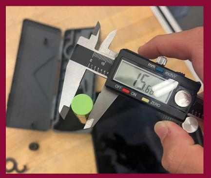
In order to create a form-fitted cap, I needed to use calipers to measure the diameter of the cap, but add a little bit to the dimensions to account for tolerancing differences when the design is set to print. After a number of test prints, I determined the perfect diameter to implement for the design.
